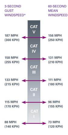
It is important to know which basis is being applied when discussing the intensity of a windstorm. Windspeed can be measured by various averaging times, such as the 3-second gust and 60-second mean. The comparison above shows the relationship between these two measurements. For example, a windspeed at the threshold of a Category 3 hurricane is 133 mph by the 3-second gust windspeed, which compares to 111 mph by the 60-second mean windspeed.
