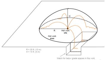
Watch for below grade spaces in the work area covered by open grating or solid grating with any openings, seams, or penetrations.
